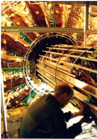
installation of optical fibres for MIPPLUG prototype
